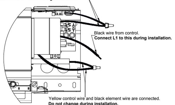
Yellow control wire and black element wire are connected. Do not change during installation.
